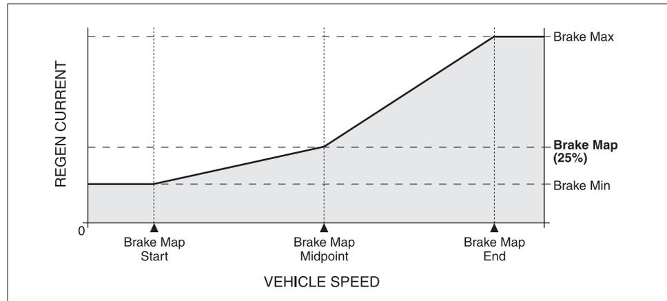
Note: Brake Map START and Brake Map END refer to the vehicle speeds at which the regen current “starts” to *increase* and “ends” *increasing*. From the operator’s perspective, however, braking begins at the point on the curve corresponding to the vehicle’s speed when braking is initiated, and then follows the curve toward “Brake Start.” The braking force is typically set to *decrease* as the vehicle slows down.
