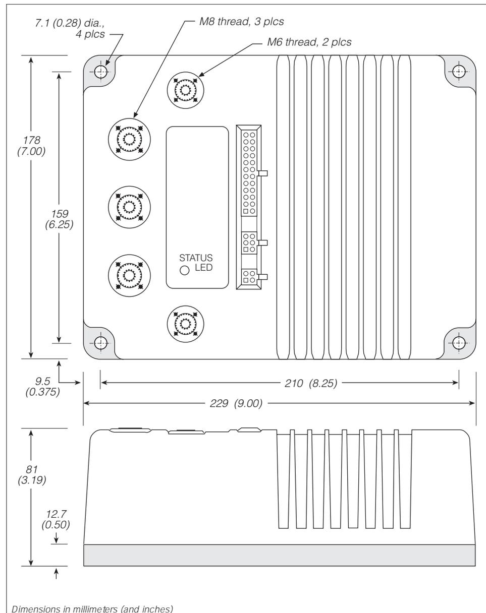
To ensure full rated power, the controller should be fastened to a clean, flat metal surface with four M6 (1/4") diameter screws, using the holes provided. Although not required, a thermal joint compound can be used to improve heat conduction from the controller heatsink to the mounting surface.
