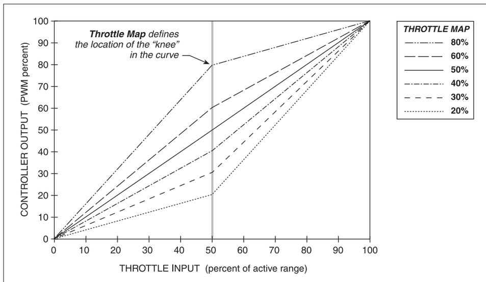
Setting THROTTLE MAP at 50% provides a linear output response to throttle position. Values below 50% reduce the controller output at low throttle settings, providing enhanced slow speed control. Values above 50% give the vehicle a faster, jumpier feel at low throttle settings.
