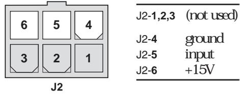
The +15V supply should only be used with the speed sensor and not to power any other external systems
